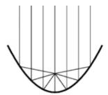
This is how a satellite dish works. Signals coming in will converge at the focus. So communications technicians place the signal pick-up at the focus point. A typical flashlight uses the same principle, but in reverse. The bulb is placed at the focus so that the light reflects off the parabolic mirror and sends the light straight ahead.
